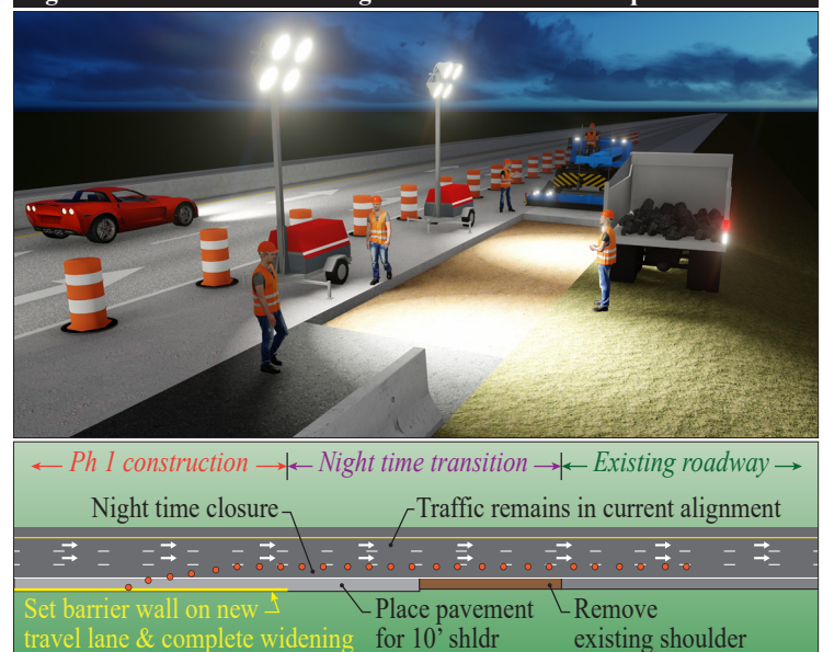
Figure 5 - MOT When Existing Material Meets S+ Requirements
